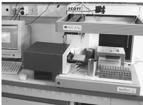
Figure 21.1. Overview of the robot analyzer intended to automatically perform a complete experiment of transmission without human intervention. The “transmission” of the digital signal was made by the mobile arm of the robot which placed the tube of water to be “informed” in an electromagnetic coil. The “imprinted” water was then mixed with plasma. Coagulation was quantified by measurement of optical density at regular intervals by the spectrophotometer visible on the left of the device. The data transmitted to the adjacent computer and the operator knew all the results including the random choice of the different “signals” only when the experiment was finished. The only steps that required human intervention were starting the device and adding reagents and consumables. The different steps performed by the robot are precisely described in the legend of Figure 23.3 of Chapter 23 ( Photo Digibio ).
